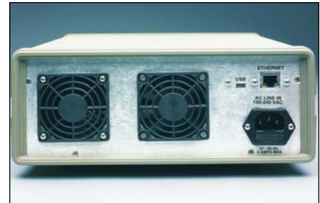
Figure 4 · Ethernet and USB interfaces are provided for connection to a computer or network.
